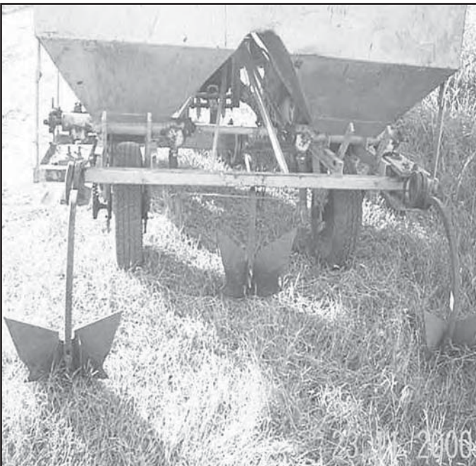
Fig. 5.5: Three spring tines, with furrower, were set at 0.9m from the centre of a frame.
