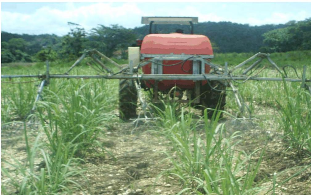
*Testing boom sprayer after setup & calibration*
