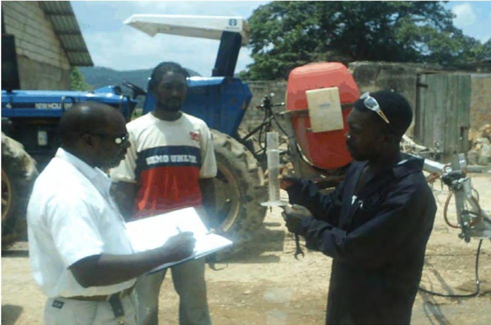
*Recording output from nozzles*
