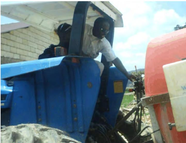
*Checking pressure gauge & adjusting pressure*
