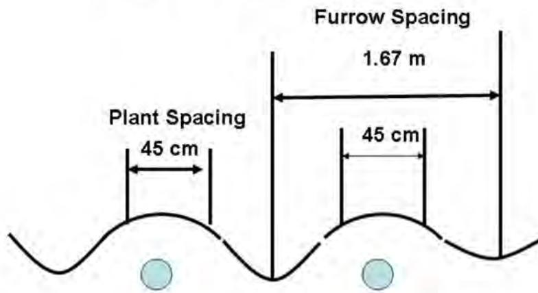
Figure 7 : Schematic Diagram of Drip Irrigation Layout
